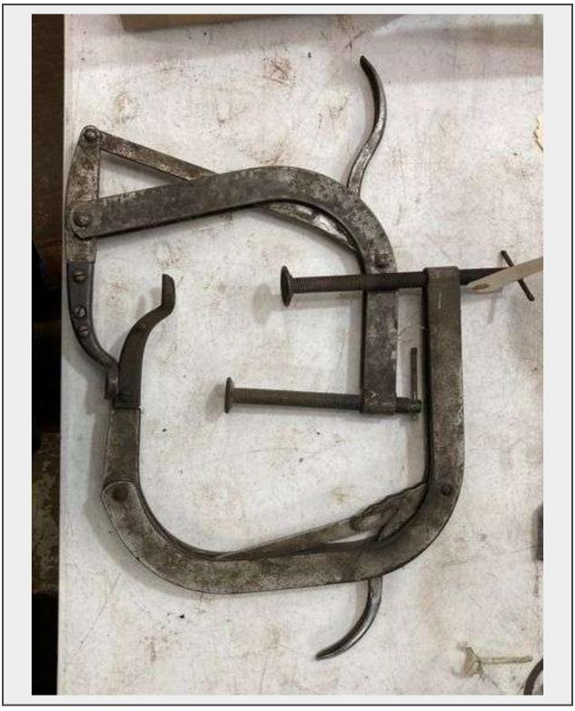
**Description** Valve spring compressors,cylinder head rebuild tools **Quantity:** 1
